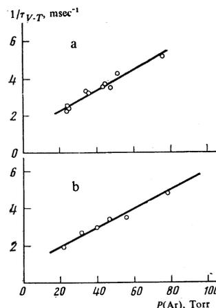
FIG. 3.  $V$ - $T$  relaxation time of  $\text{CH}_4$ ,  $\text{CH}_3\text{F}$  as a function of argon pressure for a)  $P(\text{CH}_4) = 0.12$  Torr,  $P(\text{CH}_3\text{F}) = 0.74$  Torr; b)  $P(\text{CH}_4) = 0.23$  Torr,  $P(\text{CH}_3\text{F}) = 0.36$  Torr.
