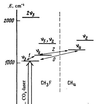
FIG. 5. The lower vibrational levels of the  $\text{CH}_3\text{F}$  and  $\text{CH}_4$  molecules.
