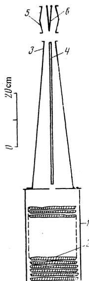
FIG. 1. Diagram of accumulator apparatus: 1—crucible; 2—plates with material; 3, 4—filter electrodes (3—ground, 4—high voltage, tube diameter 1 cm); 5, 6—collector trap electrodes; the collector 6 is made in the form of a V-shaped platinum filament of diameter 0.3 mm. The parts 1–4 are made of stainless steel.
