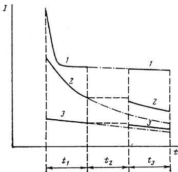
FIG. 3. Schematic representation of the expected desorption curve intervals for the desired particles in the presence of background ions. Curves 1, 2 and 3 are respectively for  $\tau \ll t_i$ ,  $\tau \sim t_i$ , and  $\tau \gg t_i$ .
