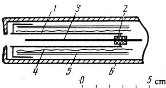
FIG. 2. Diagram of the source apparatus: 1—source crucible (tube with wall thickness  $\sim 0.5$  mm), 2—ceramic insulator, 3—needle 1 mm in diameter, 4—heater, 5—heat shields, 6—enclosure. Parts 1 and 3 are made of stainless steel and are joined by an insulating vacuum seal 2.
