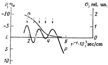
FIG. 4. Excitation cross section and degree of polarization of the  ${}^2S_{1/2}-{}^2P_{3/2}$ , radiation excited in  $\text{Sr}^+ + \text{Ar}$ , collisions vs. the reciprocal collision velocity  $v^{-1}$ . The arrows indicate the positions of the extrema of the function  $P(E)$ .
