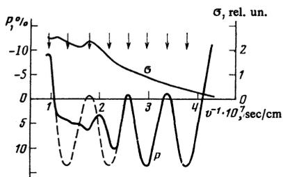
FIG. 5. Excitation cross section  $\sigma$  and degree of polarization  $P$  of the emission of the excited atom Ca ( $4^1P_1$ ) in Ca<sup>+</sup> + Kr collisions. The upper arrows indicate the positions of the extrema of the functions in the  $v^{-1}$  scale. The dashed line shows the approximate oscillations of the polarization function  $P(E)$ .
