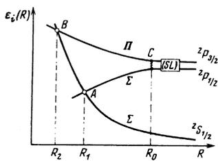
FIG. 3. Schematic behavior of the energies of the quasimolecular terms  $\varepsilon_i(R)$  as functions of the internuclear distance  $R$ .
