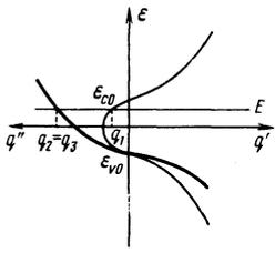
FIG. 1. Graphical solution of Eq. (4) at  $\kappa=0$  for a four-band semiconductor. The "far" roots  $q_\lambda$  ( $\lambda > 3$ ) are not shown;  $\epsilon_{c0}$  and  $\epsilon_{v0}$  are the extrema of the conduction and valence bands, respectively. The thick line separates the doubly degenerate band of heavy holes.
