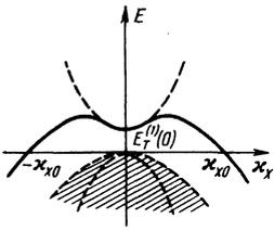
FIG. 2. Tamm subband  $E_T^{(1)}(\kappa_x)$  existing at  $R_v > 0$ . The volume states of the light and heavy holes are shaded.
