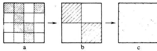
FIG. 4. Transition to an effective system of conducting squares under the scaling transformation (4) (the conducting squares are crosshatched).
