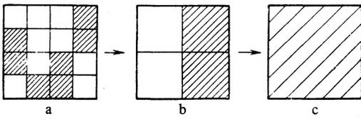
FIG. 2. Transition from an initial system of conducting squares to an effective system under the scaling transformation (3) (the conducting squares are cross-hatched); the square as a whole conducts.
