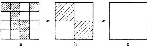
FIG. 3. Transition from an initial system of conducting squares to an effective system of conducting squares under the scaling transformation (3) (the conducting squares are crosshatched); the square as a whole does not conduct.
