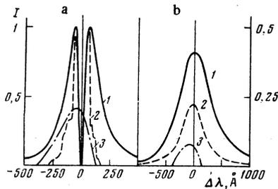
FIG. 2.  $H_\beta$  profile corresponding to the effect of ions (a) and ions and electrons (b). Curve 1—without dilution, 2—with field ionization, 3—the same according to the model in<sup>[9]</sup>;  $P=50$  atm,  $T=25\,000^\circ\text{K}$ ,  $N_e=6.3 \times 10^{18}$  cm<sup>-3</sup>. The unit of intensity is  $I=5.7 \times 10^8$  erg/Å<sup>2</sup>·cm<sup>3</sup>·sr·sec.
