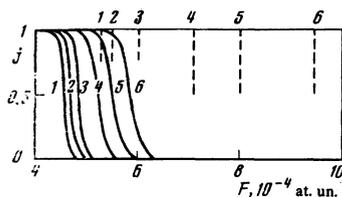
FIG. 1. Dilution coefficient for the Stark components  $(nn_1n_2m) - (n'n_1'n_2'm')$  of  $H_{\beta}$ :
