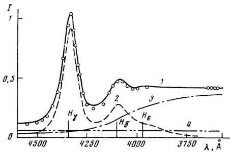
FIG. 3. Fragment of the spectrum of hydrogen plasma: 1—resultant intensity, 2—spectral lines, 3—recombinational continuum ( $n'=2$ ), 4—bremsstrahlung and recombinational continuum ( $n'=3-8$ ). Points—experiment in<sup>[1]</sup>;  $P=1$  atm,  $T=16250$  °K,  $N_e=1.7 \times 10^{17}$  cm<sup>-3</sup>,  $I=1.5 \times 10^6$  erg/Å · cm<sup>3</sup> · sr · sec.
