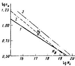
FIG. 5. Dependence of the number of the limiting level on ion density in plasma: 1—Inglis-Teller model, 2—equation (18) with  $F_{kr} = F_0$ , 3—estimate based on (23),  $\circ$ —tabulated lines with dilution  $\sim 0.5$ .
