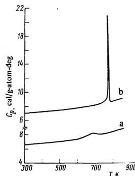
FIG. 1. Dependence of the specific heat of Pr (curve a) or Nd (curve b) on the temperature.
