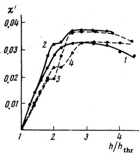
FIG. 6. Experimental dependences of  $\chi'$  on the supercriticality for  $H = H_c - 100$  Oe. The curve 1 corresponds to  $H_m = 0$  and the curves 2, 3, and 4 correspond to  $H_m = 0.14$  Oe;  $\Omega = 0.8, 1.6,$  and  $2.4$  MHz.
