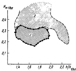
FIG. 10. The region of parametric instability of the collective oscillations.  $H = H_c - 100$  Oe,  $\Omega = 1.6$  MHz. 1) Region of strong signals of frequency  $\Omega/2$ ; 2) weak-signal region.
