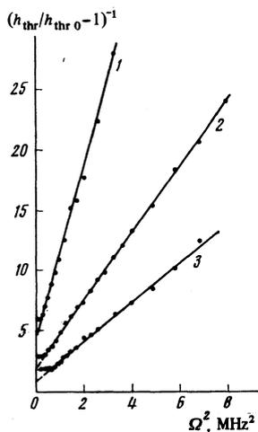
FIG. 3. Dependence of the threshold for parallel pumping on the frequency of the RF field ( $H = H_c - 100$  Oe). The curves 1, 2, and 3 correspond to  $H_m = 0.14$ , 0.21, and 0.28 Oe. In these coordinates the theory (formula (11)) predicts a straight line.
