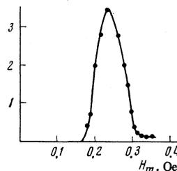
FIG. 9. Dependence of the amplitude (in arbitrary units) of the collective oscillations parametrically excited at the frequency  $\Omega/2$  on the amplitude of the RF-field pump.  $H = H_c - 100$  Oe,  $\Omega = 1.7$  MHz.
