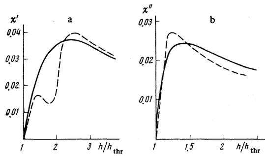
FIG. 5. a) Theoretical dependence of  $\chi'$  on the microwave-pump amplitude  $h$  for  $H_m = 0$  (the solid curve) and  $UH_m/2\gamma = 0.3$  (the dashed curve);  $2T=S$ ,  $\Omega/2\gamma = 2$  ( $H_m = 0.15$  Oe,  $\Omega = 1.6$  MHz). b) Theoretical dependence of  $\chi''$  on  $h$  for  $H_m = 0$  (the solid curve) and  $UH_m/2\gamma = 0.3$  (the dashed curve);  $2T=S$ ;  $\Omega/2\gamma = 1$  ( $H_m = 0.15$  Oe,  $\Omega = 0.8$  MHz).
