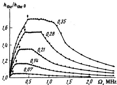
FIG. 2. Dependence of the threshold for parallel pumping on the frequency of the RF field. The numbers on the curves are the amplitudes of the RF field in oersteds. The constant magnetic field  $H = H_c - 100$  Oe. ( $H_c$  is the field corresponding to  $k = 0$ ). The arrows indicate the right-hand boundary of the low-frequency region in which the formula (11) is not applicable.
