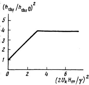
FIG. 1. Dependence of the threshold for parallel pumping on the amplitude of a modulating field of rectangular shape. In the first region the detuning  $\Delta_k = 0$ ; in the second section  $\Delta_k = \pm 2U_k H_m$ .
