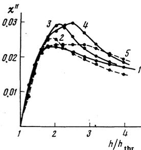
FIG. 7. Experimental dependences of  $\chi''$  on the supercriticality for  $H = H_c - 100$  Oe. For the curve 1,  $H_m = 0$ . The curves 2, 3, 4, and 5 correspond to  $H_m = 0.14$  Oe;  $\Omega = 0.8, 1.2, 1.6,$  and  $3.2$  MHz.
