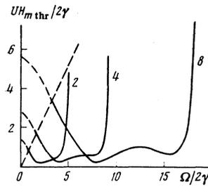
FIG. 8. Theoretical dependences (the formula (31)) of the instability threshold,  $H_{m\text{thr}}$ , for the collective oscillations on the frequency,  $\Omega$ , of the RF field. The numbers on the curves correspond to the values of the natural frequency ( $\Omega_0/2\gamma$ ) of the collective oscillations. The region of applicability of the theory is the region below the dashed line.
