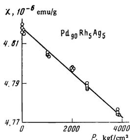
FIG. 1. Typical experimental plots of  $\chi(P)$ .
