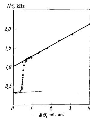
FIG. 4. Relationship between the photoconductivity signal  $\Delta\sigma_{st}$  and the reciprocal of the time constant  $1/\tau$ ,  $T = 1.7$  K,  $p_0 = 7 \cdot 10^{14}$  cm $^{-3}$ ,  $E \parallel C_3$ .
