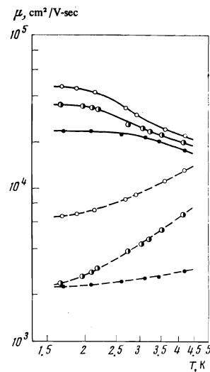
FIG. 5. The temperature dependence of the electron  $\mu_e$  (continuous line) and hole  $\mu_h$  (broken line) mobilities for samples with impurity concentrations equal to  $8 \cdot 10^{14} \text{ cm}^{-3}$  ( $\circ$ ),  $1.6 \cdot 10^{15} \text{ cm}^{-3}$  ( $\bullet$ ), and  $1.4 \cdot 10^{16} \text{ cm}^{-3}$  ( $\bullet$ ).
