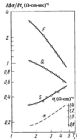
FIG. 3. Temperature dependence of the dark conductivity  $\sigma$  and the photoconductivity  $\partial\Delta\sigma/\partial t$  for different regions of the spectrum,  $p_0 = 7 \cdot 10^{14}$  cm $^{-3}$ .
