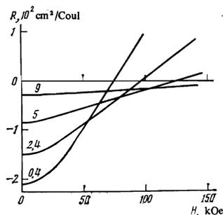
FIG. 1. Dependence of the Hall coefficient on the magnetic field intensity at various pressures (kbar),  $T = 290 \text{ }^\circ\text{K}$ .
