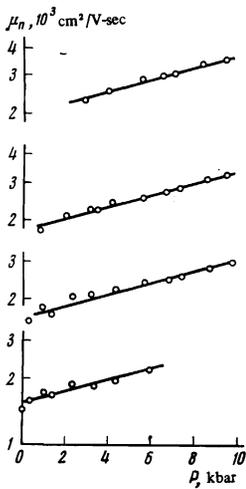
FIG. 6. Effect of pressure on the electron conductivity at various temperatures: 260, 270, 280, and 290 °K (reading downward).
