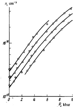
FIG. 7. Dependence of the free-carrier density on the pressure at the temperatures 290, 280, 270, and 260 °K (reading downward).
