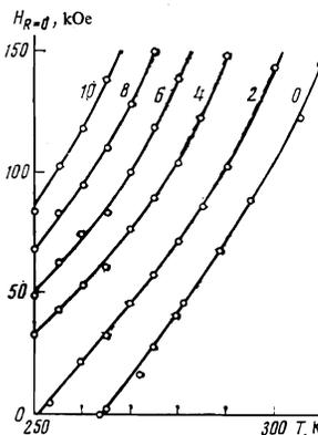
FIG. 2. Influence of temperature on the inversion field at various pressures (kbar).
