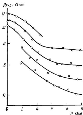
FIG. 3. Dependence of the magnetoresistance in the inversion fields on the pressure at the temperatures 290, 280, 270, 260, and 250 °K (reading downward).
