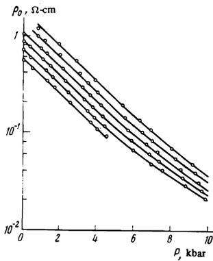
FIG. 4. Effect of pressure on the resistivity of the sample at the temperatures 250, 260, 270, 280, 290, and 300 °K (reading downward).
