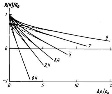
FIG. 5. Dependence of the relative Hall coefficient on the relative magnetoresistance at various pressures (kbar).
