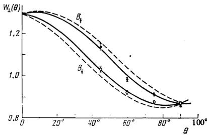
FIG. 3. Angular correlation function of  $\alpha$ - $e$  cascade in Pu with opposite directions of the magnetic field. The dashed curves show the same functions but corrected for the stray magnetic field.
