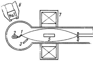
FIG. 1. Diagram of experimental setup: 1—iron-foil source, 2—electromagnet winding, 3—detector, 4—Si(Li) conversion-electron detector, 5—lead shield against fragments,  $\alpha$  particles, and  $\gamma$  quanta, 6—scintillation  $\gamma$  detector, 7—coil of short magnetic lens.
