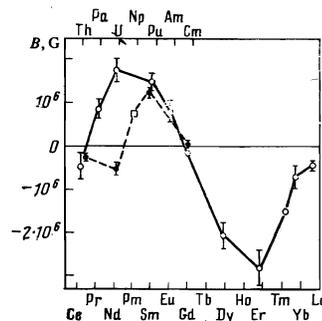
FIG. 4. Comparison of the effective magnetic fields in an iron matrix for lanthanides (solid curve) and actinides (dashed). The small square marks the value of the field for neptunium, recalculated from the known value of the field in nickel.
