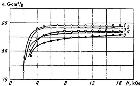
FIG. 1. Magnetization curves of MnSb alloy at room temperature 294°K and at various pressures (kbar): 1—10<sup>-3</sup>; 2—4.1; 3—5.6; 4—6.7; 5—8.2.
