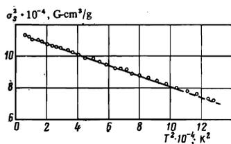
FIG. 4. Dependence of  $\sigma_s^2$  on  $T^2$  of the alloy MnSb at atmospheric pressure.
