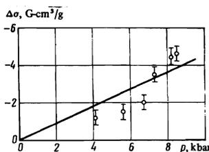
FIG. 2. Variation of the magnetization of MnSb at  $T = 294^\circ\text{K}$  with changing pressure.
