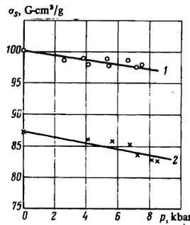
FIG. 3. Pressure dependence of the spontaneous magnetization of the alloy MnSb at  $T_1 = 83^\circ\text{K}$  (curve 1) and  $T_2 = 294^\circ\text{K}$  (curve 2).
