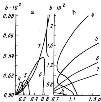
FIG. 4. The spectrum of electromagnetic waves in a metallic ferromagnet. The number of the curve is the same as the value of  $n$  for which this curve is constructed. The interval of change of  $\rho$  is broken into two parts. On one of them (a), the scale along the ordinate is 20 times greater than on the other (b). The curve shown by the dashed lines is determined by the expression (18).
