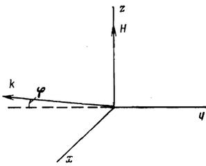
FIG. 2. System of coordinates. The  $z$  axis is perpendicular to the plane passing through the magnetic field vector  $H$  and the wave vector  $k$ . The angle  $\varphi \ll 1$ .
