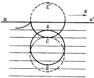
FIG. 1. Trajectories of electrons in a magnetic field close to the surface of the metal. The wave vector of the electromagnetic wave, propagating perpendicular to the surface of the metal  $aa'$ , makes an angle with the direction of the magnetic field that is close to  $\pi/2$ . The system of parallel lines represent the planes of equal phase of the wave. The  $x$  axis is parallel to the corresponding axis of the system of coordinates (Fig. 2).
