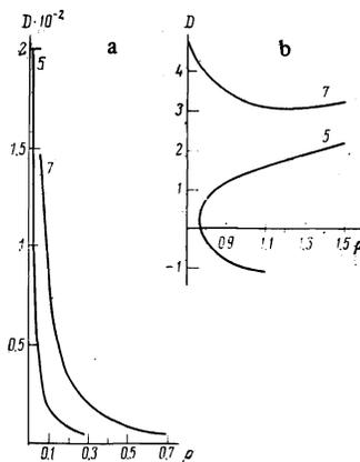
FIG. 5. The dependence on  $\rho$  of the coefficient of polarization of the electric field in the electromagnetic wave. The number of the curve is the same as the value of  $n$  for which this curve is constructed. At  $\rho < 0.7$  (a) and at  $\rho \geq 0.7$  (b), the scales along the ordinate axes is chosen differently.
