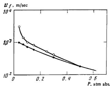
FIG. 6. Discharge velocity in a tube of diameter 6.5 mm,  $\circ$ — $H = 0$ ;  $\bullet$ — $H = 9.3$  kOe.
