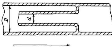
FIG. 4. Schematic diagram of the "trap."  $D/d \approx 2$  for tubes with different diameters. The arrow indicates the direction of the discharge motion.
