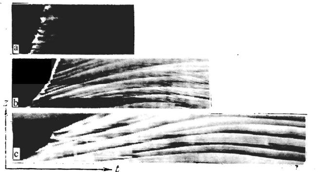
FIG. 3. Streak photograph of the discharge in argon: a)  $P = 1.0$  atm abs.,  $W = 1200$  W; tube diameter 20 mm; b)  $P = 0.5$  atm abs.,  $W = 1200$  W,  $\varnothing 6.5$  mm; c)  $P = 2.6$  atm abs.,  $W = 1200$  W,  $\varnothing 6.5$  mm. Slit dimension  $4 \times 20$  mm.
