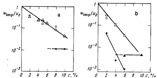
FIG. 9. Dependence of the discharge velocity in a mixture of argon with various impurities on the impurity concentration  $c$  at different pressures: a) 0.1 atm abs., b) 1.0 atm abs., circles—hydrogen, triangles—nitrogen. The light and dark symbols correspond to the fast and slow discharge-propagation mechanisms. Tube diameter 20 mm,  $W = 1200$  W.
