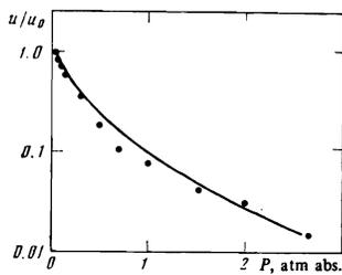
FIG. 7. Discharge velocity in a tube of 6.5 mm diameter. Solid line—calculation, points—experiment.
