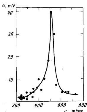
FIG. 8. Dependence of the pressure-pickup signal amplitude on the microwave discharge velocity.  $P = 1.0$  atm abs. Tube diameter 20 mm.
