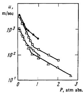
FIG. 1. Dependence of the microwave-discharge velocity on the pressure in argon for tubes of various diameters at different power-supply levels: ●— $\varnothing$  20 mm,  $W=1200$  W; □— $\varnothing$  9.5 mm,  $W=1200$  W; △— $\varnothing$  6.5 mm,  $W=1200$  W; ○— $\varnothing$  20 mm,  $W=500$  W.
