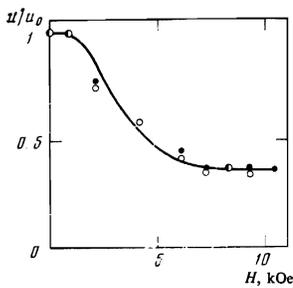
FIG. 5. Dependence of the discharge velocity in argon on the magnetic field,  $P = 4 \times 10^{-2}$  atm abs.  $\circ$ —tube diameter 6.5 mm,  $\bullet$ —9.5 mm,  $\bullet$ —6.5 and 9.5 mm.
