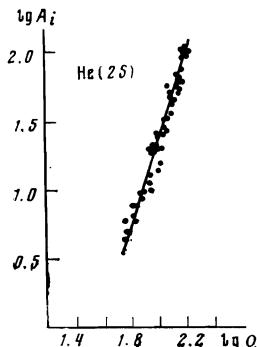
FIG. 2. Probe signal amplitude  $A_i$  as a function of energy  $Q$  per radiation pulse (logarithmic scales).
