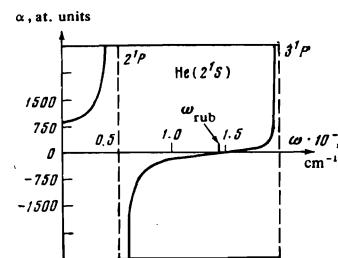
FIG. 10. Dynamic polarizability  $\alpha$  of the helium atom in the  $2^1S$  state as a function of frequency (theoretical calculation from<sup>[11, 12]</sup>).  $\omega_{\text{rub}}$  is the ruby laser frequency.
