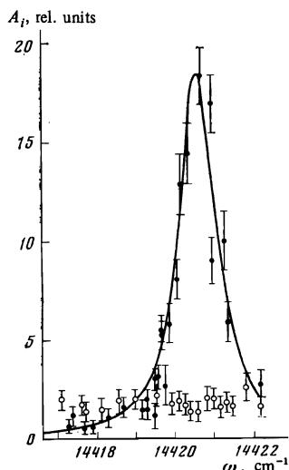
FIG. 4. Probe-signal amplitude  $A_i$  as a function of the frequency  $\omega$  at a constant laser intensity: ●—plane polarization; ○—circular polarization.
