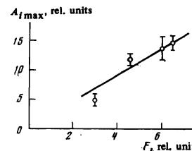
FIG. 9. Probe-signal amplitude at resonance  $A_f, \text{max}$  as a function of the radiation intensity  $F$ .
