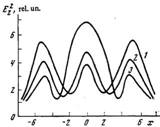
FIG. 7. Theoretical plots of the density  $E_2^2$  of the reflected wave of a ring laser vs the generation frequency  $x$  at different gas absorption coefficients: 1 -  $G_{0-}/G_0 = 10^{-3}$ ; 2 -  $G_{0-}/G_0 = 2 \cdot 10^{-3}$ ; 3 -  $G_{0-}/G_0 = 5 \cdot 10^{-3}$ .
