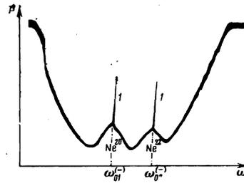
FIG. 5. Oscillograms illustrating the onset of high- $Q$  self-oscillation resonances in the case of hyperfine splitting of the line of a weakly absorbing gas.
