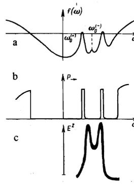
FIG. 6. Formation of high- $Q$  nonlinear-absorption resonances due to the competition of the waves of the ring laser in the presence of two neighboring spectral components in the line of a strongly absorbing gas.
