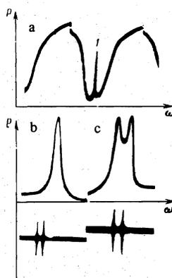
FIG. 2. Oscillograms illustrating the splitting of the nonlinear absorption resonance of methane in a magnetic field: a) Overall view of the scanning zone (1—methane resonance), b) shape of the resonance at small scanning amplitudes, c) splitting of the resonance in a magnetic field  $H = 210$  Oe. The distance between the frequency markers is 100 kHz.
