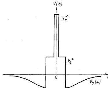
FIG. 1. Shape of the effective potential  $V(x)$ . The half-width of the humps  $V_e^<$  and  $V_i^<$  at the center of the Teller well  $V_0(x)$  is  $\Delta_e$  and  $\Delta_i$ , respectively.
