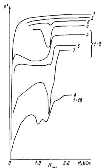
FIG. 1. Passage of the high-frequency power through a resonator with the sample.  $P'$ —power fed to the input of the receiver. Curves 1–8 correspond to the following values of the damping of the input attenuator: 1)—46, 2)—44.2; 3)—43.5; 4)—39.35; 5)—28.1; 6)—23.8; 7)—16.2; 8)—7.65 dB.
