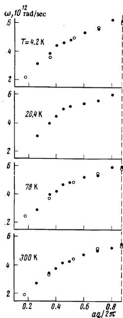
FIG. 1. Dispersion of transverse phonons in lead in the [111] direction at different temperatures: ●—our data, ○—data of [5]. The dashed line shows the band boundary.
