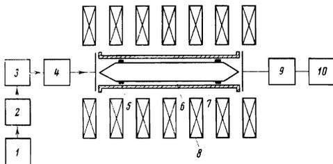
FIG. 1. Experimental setup: 1—generator, 2—decoupler, 3—measuring line, 4—"tourniquet" junction, 5—electrodes, 6—discharge tube, 7—dismantlable waveguide section, 8—multi-sector solenoid, 9—detector section, 10—matched load.
