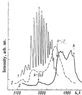
FIG. 4. Generation (1) and spontaneous emission (2) spectra of a streamer discharge in CdS at  $T = 80^\circ\text{K}$ . The photoluminescent spectrum of the same sample (3) is shown for comparison.
