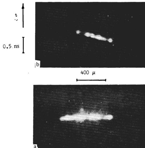
FIG. 5. Streak photograph of the light-generation region in a streamer without a time scan (a) and with a time scan (b).
