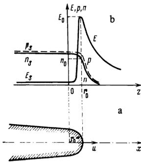
FIG. 6. Picture of streamer moving in the direction of the X axis (a) and the distribution of the nonequilibrium-carrier density and of the electric-field intensity along the streamer axis (b).
