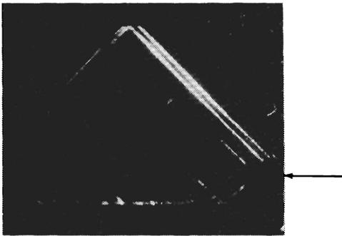
FIG. 2. Generation of light in streamer discharges in CdS plates at  $T = 80^\circ\text{K}$ . The arrow shows the point where the pulse voltage was applied. The length of the double track is 0.8 cm.
