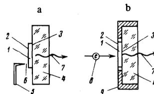
FIG. 1. Excitation of streamer discharges by applying electric-pulses through a discharge gap (a) and by charging the crystals with an electron beam in vacuum (b): 1—investigated crystal, 2, 3—dielectric mirrors, 4—sapphire or glass substrate, 5—high-voltage electrode, 6—gap filled with liquid dielectric, 7—investigated radiation, 8—electron beam, 9—metal frame.
