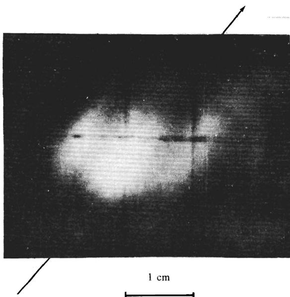
FIG. 3. Photograph of the angular divergence of the radiation generated by an individual track at a distance of 3 cm from the CdS plate. The arrow indicates the direction along the track axis.
