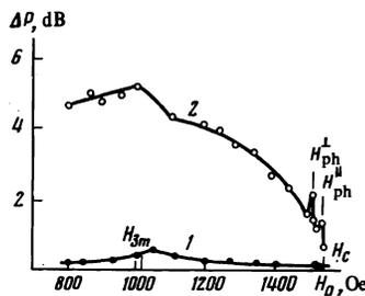
FIG. 4. Gap  $\Delta P$  between the power at which the low-frequency self-modulation of the magnetization sets in and the threshold power of the parametric instability in the case of parallel pumping, as a function of the constant magnetic field  $H_0$  for samples of 1.02 mm diameter (curve 1) and 0.18 mm diameter (curve 2);  $H_0 \parallel [111]$ .
