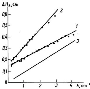
FIG. 2. Dependence of the spin-wave damping parameter  $\Delta H_k$  on the wave vector  $k$  for YIG spheres of diameter 1.02 mm (curve 1) and 0.18 mm (curve 2). Line 3 was obtained by subtracting curve 1 from curve 2;  $H_0 \parallel [111]$ .
