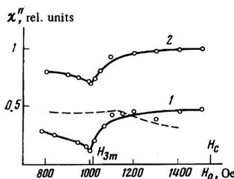
FIG. 3. Dependence of the imaginary part of the nonlinear susceptibility  $\chi''$  in parallel pumping on the constant magnetic field  $H_0$  at excess of the pump over the threshold level  $P/P_p = 1$  dB (curve 1) and  $P/P_p = 3$  dB (curve 2). The sample is a YIG sphere of 0.18 mm diameter;  $H_0 \parallel [111]$ . Dashed curve—experimental dependence for  $\chi''$  on  $H_0$  for a YIG sphere of 2.11 mm diameter;  $H_0 \parallel [111]$ ,  $P/P_p = 1$  dB.<sup>[8]</sup>
