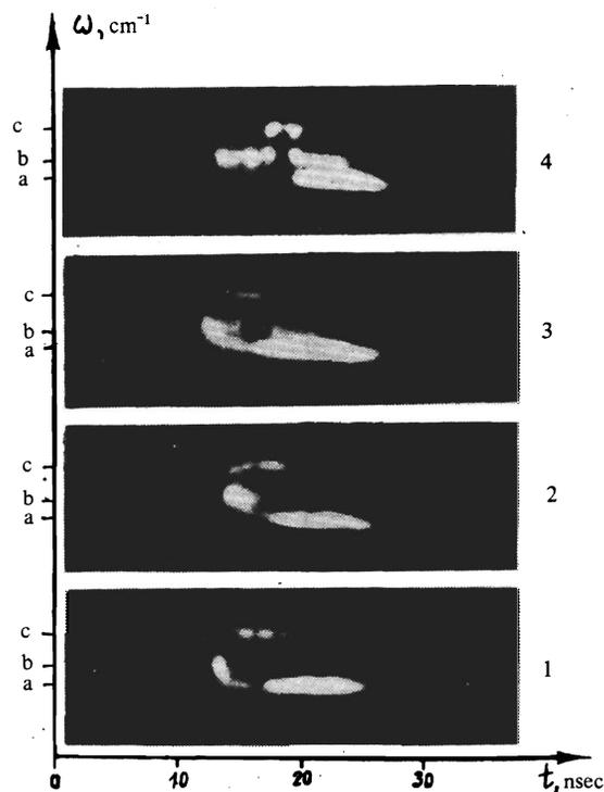
FIG. 3. Spectrochronograms of the stimulated processes in potassium vapor in the case of excitation by resonance radiation. The "backward" scheme. Temperature of the potassium vapor: 1) 305 °C, 2) 315 °C, 3) 320 °C, 4) 340 °C; a) incident radiation, b) the three-photon scattering radiation, c) the SERS radiation.
