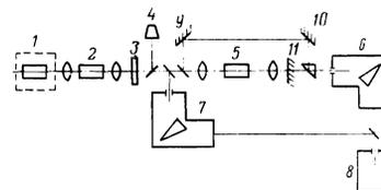
FIG. 1. Diagram of the experimental setup: 1) ruby laser with Q switching; 2) cuvette with organic liquid and of length  $l=20$  cm; 3) FS-7 filter; 4) calorimeter; 5) cuvette with potassium; 6), 7) ISP-51 spectrographs; 8) FER-2 photoelectronic detector; 9)–11) 100-percent dielectric mirrors.
