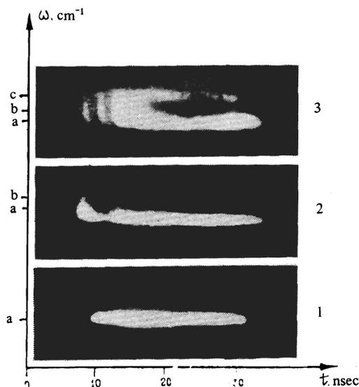
FIG. 2. Spectrochronograms of the stimulated processes in potassium vapor in the case of excitation by resonance radiation. The "direct" scheme. Temperature of the potassium vapor: 1) 190 °C, 2) 300 °C, 3) 340 °C; a) incident radiation, b) the three-photon scattering radiation, c) the SERS radiation.
