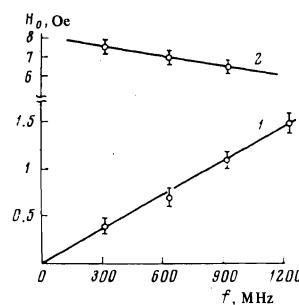
FIG. 6. Frequency dependences of the position of the  $dR/dH$  maximum on the magnetic field axis plotted for a cylindrical sample: 1)  $T=3.68$  °K, superconducting state; 2)  $T=3.73$  °K, normal state.
