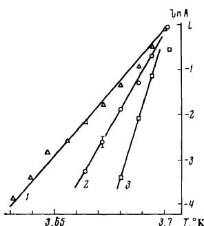
FIG. 5. Anisotropy of the temperature dependence of the amplitude of the  $dR/dH$  peak of a disk with  $n \parallel [110]$ : 1)  $H \parallel [001]$ ; 2) angle between  $H$  and  $[001]$  equal to  $45^\circ$ ; 3)  $H \perp [001]$ .
