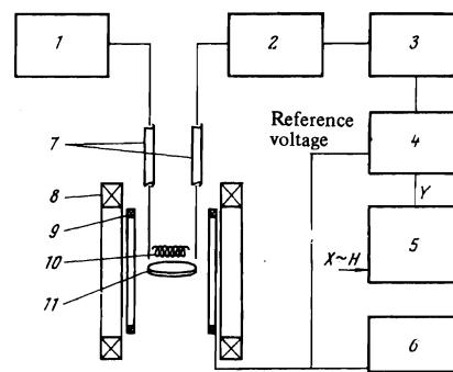
FIG. 1. Block diagram of the apparatus for investigating the dependence of  $dR/dH$  on the magnetic field in the frequency range 300–1200 MHz: 1) oscillator (300–1200 MHz); 2) receiver (200–1200 MHz); 3) amplifier (30 Hz); 4) phase-sensitive detector; 5) X-Y plotter; 6) oscillator (30 Hz); 7) coaxial lines; 8) Helmholtz coils; 9) modulation coils; 10) resonator helix; 11) sample.
