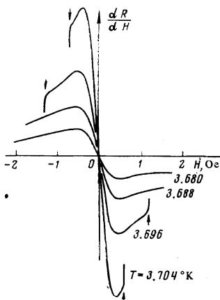
FIG. 2. Dependences of  $dR/dH$  of a cylindrical sample of tin on the magnetic field at 658 MHz. Here,  $H \parallel h$  and it is parallel to the cylinder axis.
