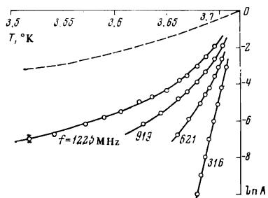
FIG. 3. Temperature dependences of the amplitude of the  $dR/dH$  peak of a cylindrical sample at four frequencies. The ordinate is the natural logarithm of  $A = dR(H_0)/dH - dR(0)/dH$ , where  $H_0$  is the position of the  $dR/dH$  maximum. The dashed curve is the dependence  $R_s(T)/R_N(T_d)$  obtained by Pippard<sup>[5]</sup> at 1200 MHz.
