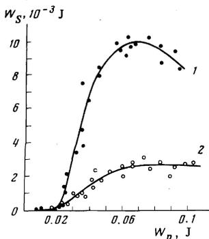
FIG. 5. Dependence of the SRS Stokes-component energy on the pump energy. 1) "Axial" part of the SRS Stokes component, corresponding to curve 1 of Fig. 4a. 2) "Conical" part of the Stokes component of the SRS corresponding to curve 2 of Fig. 4a.
