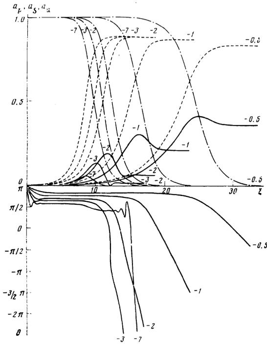
FIG. 1. Plots of  $a_a$  (solid curve),  $a_p$  (dash-dot), and  $a_s$  (dashed), and  $\theta$  against  $\xi$  at  $\delta = -7, -3, -2, -1$ , and  $-0.5$ , obtained for the ratio  $\omega_{21}/\omega_p = 0.22$  and for the initial values  $a_a|_{\xi=0} = 10^{-6}$ ,  $a_s|_{\xi=0} = 10^{-3}$ ,  $a_p|_{\xi=0} = 1$ , and  $\theta|_{\xi=0} = \pi$ . It is assumed that  $r_1 = r_2 = 1$ .
