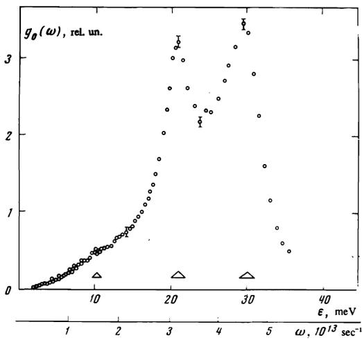
FIG. 1. Phonon spectrum of vanadium. The triangles indicate the resolution of the apparatus.
