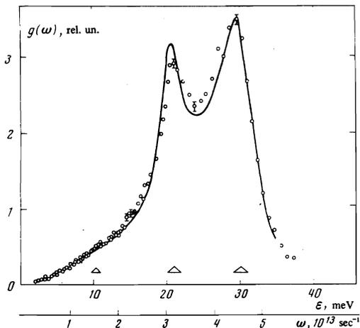
FIG. 2. Spectrum of the vibrational excitations of the alloy  $V_{0.943}Ta_{0.057}$ . Points—VTa spectrum, solid curve—V spectrum.
