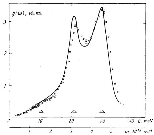
FIG. 3. Spectrum of vibrational excitations of the alloy  $V_{0.945}W_{0.055}$ . Points—VW spectrum, solid curve—V spectrum.
