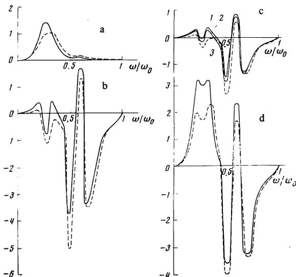
FIG. 4. Calculated values of the functions of the impurity crystals: a)  $K_{\text{imp}}$ ; b)  $\Delta K_{\text{latt}}$ ; d)  $\Delta g$  for VW (solid curve— $\gamma_0 = \gamma_1$ ; dashed— $\gamma_0 = 1.4\gamma_1$ ); c)  $\Delta \sigma/cRN_T$ ; 1—VTa ( $\gamma_0 = \gamma_1$ ), 2—VW ( $\gamma_0 = \gamma_1$ ), 3—VW ( $\gamma_0 = 1.4\gamma_1$ ).
