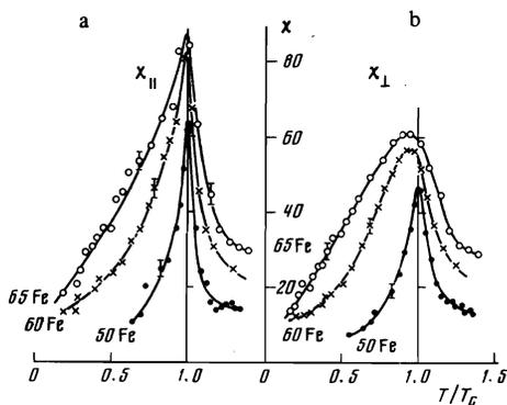
FIG. 5. Temperature dependences of the longitudinal  $\chi_{\parallel}$  and transverse  $\chi_{\perp}$  components of the magnetic susceptibility tensor of iron-nickel alloys.
