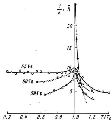
FIG. 6. Temperature dependences of the dimensions of the longitudinal spin correlation in iron (●), nickel (+),<sup>[5]</sup> and Fe-Ni alloys.
