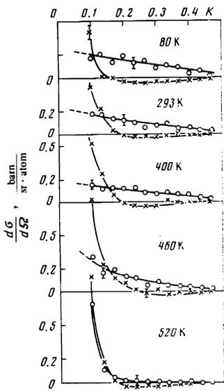
FIG. 4. Angular dependences of the difference cross sections obtained at various temperatures for the 65Fe-35Ni alloy ( $K = 2\pi\lambda^{-1}\sin\theta$ ): ○)  $(d\sigma/d\Omega)_{0-||}$ ; ×)  $(d\sigma/d\Omega)_{0-\perp}$ .
