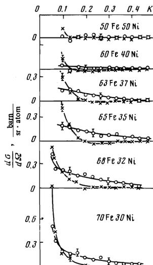
FIG. 3. Angular dependences of the difference cross sections obtained at room temperature for various alloys ( $K = 2\pi\lambda^{-1}\sin\theta$ ):  $\circ$ )  $(d\sigma/d\Omega)_{0-\parallel}$ ;  $\times$ )  $(d\sigma/d\Omega)_{0-\perp}$ .
