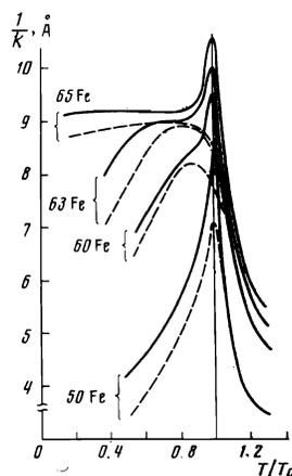
FIG. 7. Comparison of the temperature dependences of the dimensions of longitudinal and transverse spin correlations in Fe-Ni alloys. The continuous curves represent  $k_{\parallel}^{-1}$  and the dashed curves  $k_{\perp}^{-1}$ .
