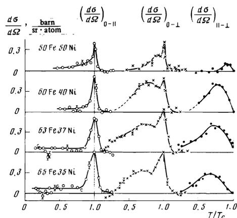
FIG. 2. Temperature dependences of the difference scattering cross sections obtained for various alloys at the angle  $2\theta = 1^{\circ}10'$ .
