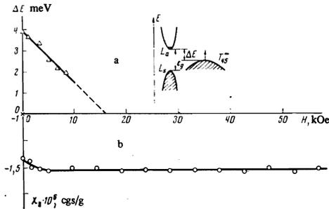
FIG. 5. a) Gap  $\Delta\epsilon$  in the spectrum of the alloy  $\text{Bi}_{0.924}\text{Sb}_{0.076}$  (sample No. 10) vs. the magnetic field  $H \parallel C_3$ . The arrow in the insert indicates the motion of the edge of the band in a magnetic field at  $H \parallel C_3$ . b) Differential magnetic susceptibility  $\chi_{\perp}$  of the same alloy at  $H \parallel C_3$ ,  $T = 4.2^\circ\text{K}$ .
