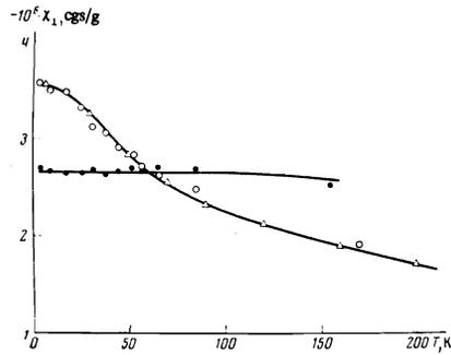
FIG. 4. Temperature dependences of the differential magnetic susceptibility  $\chi_{\perp}$  of sample No. 10 for two values of the magnetic field  $H \parallel C_2$ :  $\circ$ —2.4 kOe,  $\bullet$ —47.2 kOe;  $\triangle$ —data of [8] for  $\chi_{\perp}(0)$  of the alloy  $\text{Bi}_{0.92}\text{Sb}_{0.08}$ .
