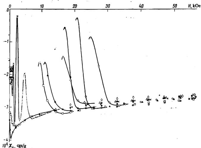
FIG. 2. Plots of the differential magnetic susceptibility  $\chi_{\perp}$  vs. the magnetic field  $\text{H}||\text{C}_1$  at  $4.2^{\circ}\text{K}$  for the samples:  $\circ$ —No. 1,  $\circ$ —2,  $\bullet$ —3,  $\Delta$ —4,  $\blacktriangle$ —5,  $\square$ —6,  $\times$ —8,  $\diamond$ —9,  $\blacklozenge$ —10.
