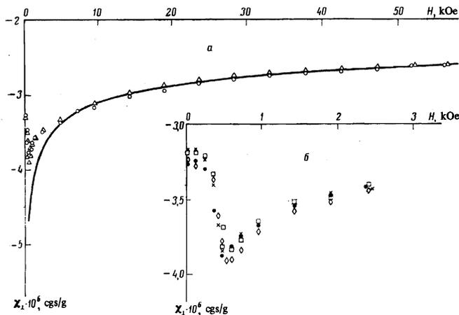
FIG. 1. Plots of the differential magnetic susceptibility  $\chi_{\perp}$  of the alloy  $\text{Bi}_{0.924}\text{Sb}_{0.076}$  (sample No. 12) vs. the magnetic field at  $T=4.2^{\circ}\text{K}$ . a)  $\text{H}||\text{C}_1$  ( $\circ$ ) and  $\text{H}||\text{C}_2$  ( $\Delta$ ); b)  $\text{H}||\text{C}_2$  at various modulation frequencies:  $\bullet$ —21.9,  $\circ$ —36.4,  $\diamond$ —61.9,  $\square$ —94.1 Hz.
