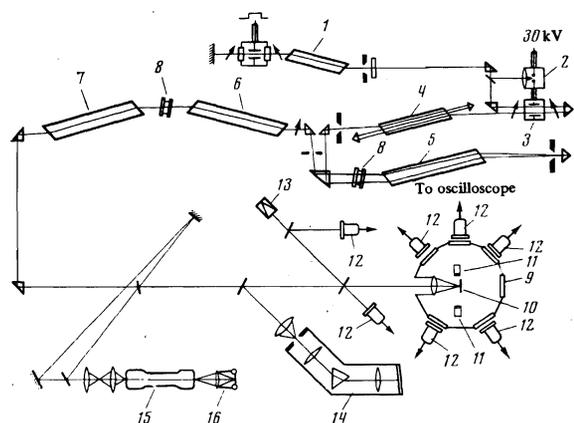
FIG. 1. Experimental setup: 1—neodymium laser Q-switched with a Kerr cell, 2—discharge gap with laser ignition, 3—shaping Kerr cell, 4—three-pass amplifier, 5—two-pass amplifier, 6, 7—one-pass amplifiers, 8—cells with saturable filters, 9—vacuum chamber, 10—target, 11—x-ray detectors, 12—coaxial photocells connected to oscilloscope, 13—calorimeter, 14—prism spectrograph, 15—photoelectric recorder (FER-2), 16—photographic camera.
