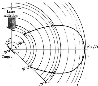
FIG. 3. Typical directivity pattern of reflected radiation in a plane perpendicular to the laser-radiation polarization, for the case of incidence of the light beam on the target at  $45^\circ$ , at a flux density  $q \approx 7 \times 10^{13}$  W/cm<sup>2</sup> (the arcs drawn through the experimental points indicate the apertures of the recording photocells).
