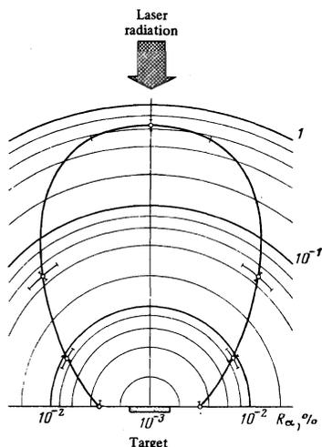
FIG. 2. Typical directivity pattern of reflected radiation in a plane perpendicular to the polarization vector of the laser-radiation polarization, for the case of normal incidence of the light beam on the target at a flux density  $q \approx 6 \times 10^{13}$  W/cm<sup>2</sup> (the arcs drawn through the experimental points indicate the aperture of the registering photocells).
