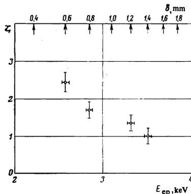
FIG. 6. Dependence of the degree anisotropy  $\zeta$  of the x rays on the end-point energy  $E_{ep}$  of the transmission of a beryllium filter (corresponds to attenuation of the radiation by a factor  $10^2$  in a filter of thickness  $\delta$ ) for an aluminum target,  $q = 5 \times 10^{13}$  W/cm<sup>2</sup>.
