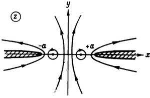
FIG. 1. Superconducting bridge with two quantum vortices.
