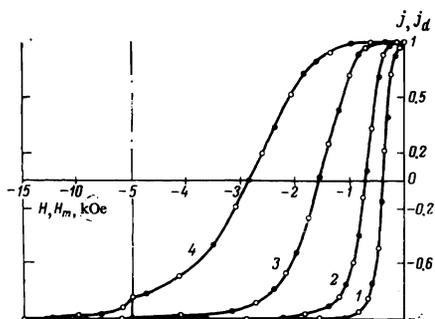
FIG. 5. Demagnetizing branches of limiting hysteresis loops  $j(-H)$  ( $\circ$ ) and corresponding remanent-magnetization curves  $j_d(-H_m)$  ( $\bullet$ ) of textured specimens of powders 1-4.  $j$  and  $j_d$  are in relative units; the vertical dot-dash line indicates a change of scale.
