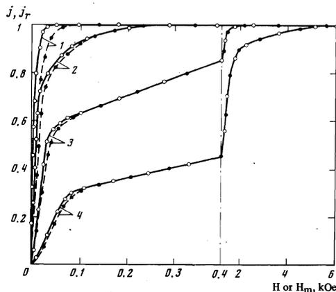
FIG. 2. Magnetization curves  $j(H)$  (○) and remanent-magnetization curves  $j_r(H_m)$  (●) of textured specimens of powders 1-4. Here and below, the numbers on the curves correspond to the numbers of the powders in the table;  $j$  and  $j_r$  are in relative units; the vertical dot-dash line indicates a change of scale.
