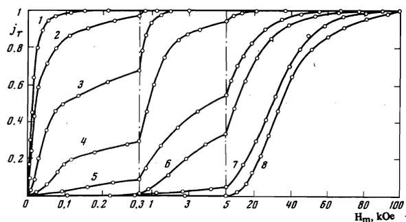
FIG. 3. Remanent-magnetization curves of isotropic specimens of powders 1-8.  $j_r$  is in relative units; the vertical dot-dash line indicates a change of scale.
