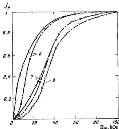
FIG. 4. Remanent-magnetization curves of isotropic specimens of powders 6-8, measured with initial thermally demagnetized ( $\circ$ ) and remanently magnetized ( $\times$ ) states of the particles.  $j_r$  is in relative units.
