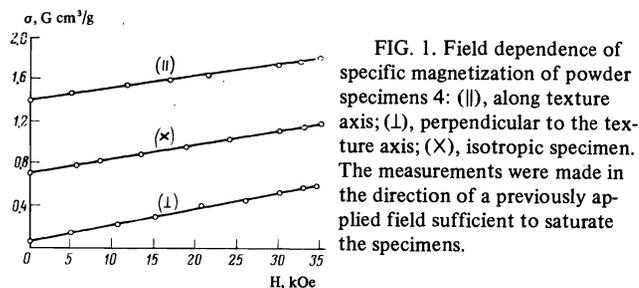
FIG. 1. Field dependence of specific magnetization of powder specimens 4: (ii), along texture axis; (1), perpendicular to the texture axis; (x), isotropic specimen. The measurements were made in the direction of a previously applied field sufficient to saturate the specimens.
