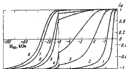
FIG. 6. Remanent-magnetization curves of isotropic specimens, corresponding to limiting hysteresis loops.  $j_d$  is in relative units; the vertical dot-dash line indicates a change of scale.
