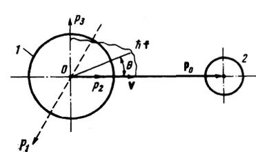
FIG. 5. Illustrating the calculation of  $\delta B$  for interband transitions between the anomalous and main bands: 1—the surface  $\epsilon_{1p} = p^2/2m_1$ ; 2—the surface  $\epsilon_{2p} = \epsilon_c + (p - p_0)^2/2m_2$ . The dislocation axis (dashed) is perpendicular to the vector  $\mathbf{p}_0$ .
