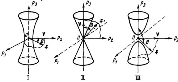
FIG. 2. Different variants of dislocation motion when the neck is broken in case B: I—dislocation axis parallel to the  $p_3$  axis of the neck; II—dislocation axis perpendicular and the velocity  $V$  is parallel to the neck axis; III—dislocation axis and velocity perpendicular to the neck axis (the dislocation axis is shown dashed).
