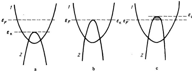
FIG. 4. Onset of hole band in a phase transition of order  $2^{1/2}$ : a)  $z = \epsilon_F - \epsilon_c > 0$ ; b)  $z = 0$ ; c)  $z < 0$ ;  $1 - \epsilon_{1p} = p^2/2m_1$ ;  $2 - \epsilon_{2p} = \epsilon_c - p^2/2m_2$ . The dashed lines show the hole band.
