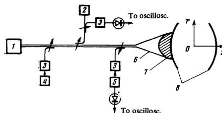
FIG. 1. Diagram of setup: 1—magnetron, 2—VI-1 power meter, 3—attenuator, 4—klystron oscillator, 5—flow-through resonator, 6—horn, 7—teflon lens, 8—open resonator.
