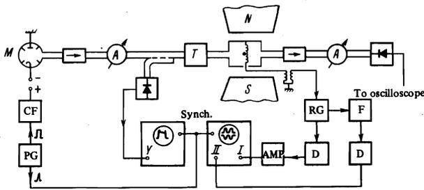
FIG. 1. Experimental setup: M—magnetron, CF—cathode follower, PG—rectangular-pulse generator, A—attenuator, T—impedance transformer, RG—radio-frequency generator, F—frequency meter, D—detector, AMP—tuned amplifier
