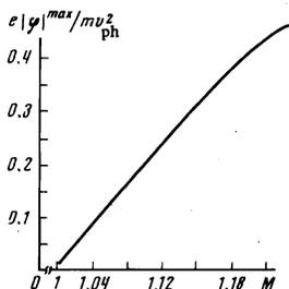
FIG. 1. Dispersion relation (amplitude as function of Mach number) for a two-dimensional solitary charge density wave.
