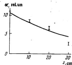
FIG. 6. Damping of the amplitude of a solitary wave in the plasma;  $z$ —distance from the exciting grid.
