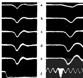
FIG. 5. Oscillograms of a charge density soliton plotted at different distances from the exciting grid: a—when there is no beam, b to e—for different values of the beam velocity, e—form of the pulse produced at the grid and time marks.
