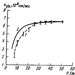
FIG. 4. The phase velocity of the solitary wave as function of the magnetic field strength for constant amplitude of the exciting signal: 1—experiment, 2—theory.
