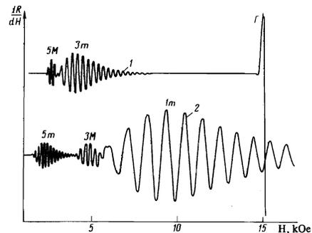
FIG. 5. Calculated plots of the derivative of the surface resistance against the magnetic field in the case of positive (curve 1) and negative (curve 2) polarization at a frequency  $f_0 = 200$  kHz and a plate thickness  $d = 0.50$  mm.
