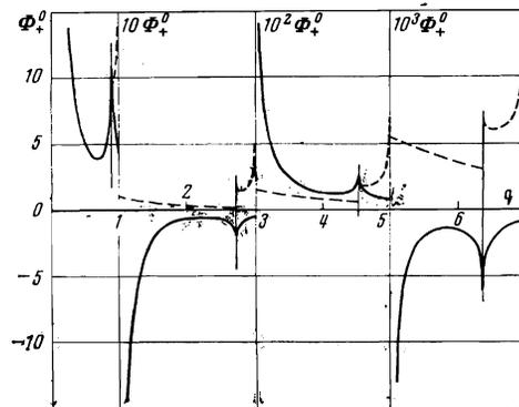
FIG. 2. Dependence of the real (solid curves) and imaginary (dashed curves) parts of the function  $\Phi_{+}^0$  on the reduced wave number  $q$ . The ordinate scale is different in different regions of  $q$ .
