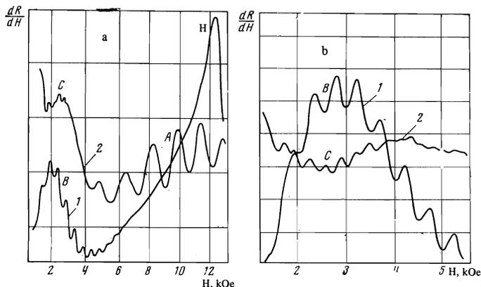
FIG. 6. Plots of  $dR_{\pm}/dH$  against the magnetic field for samples of thickness  $d = 0.31$  mm: a—frequency  $f = 170$  kHz, b—510 MHz;  $T = 4.2^\circ\text{K}$ . Curves 1 and 2 correspond to polarization plus and minus, respectively. The plots for equal frequencies were drawn at equal gains.
