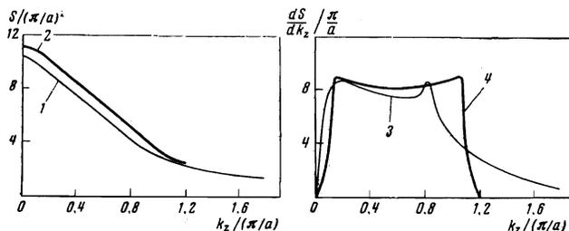
FIG. 1. Plots of the area (curves 1 and 2) and of the derivative of the area (curves 3 and 4) of the cross section of the Fermi surface of aluminum;  $k_z \parallel [100]$ .
