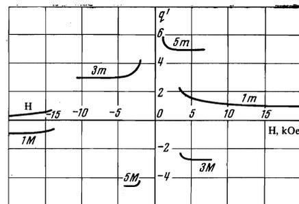
FIG. 3. Dependence of the real parts of  $q$  on the magnetic field intensity at  $f_0 = 200$  kHz. The curve H corresponds to the helicon; the curves 1M, 3M, and 5M correspond to multiple dopplerons due to the minimum of  $\partial S/\partial k_z$ ; the curves 1M, 3M, and 5M correspond to multiple dopplerons due to the maximum of  $\partial S/\partial k_z$ .
