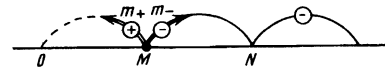
FIG. 2. Carrier trajectory at metal-vacuum interface. An electron is converted into a hole at the point M.
