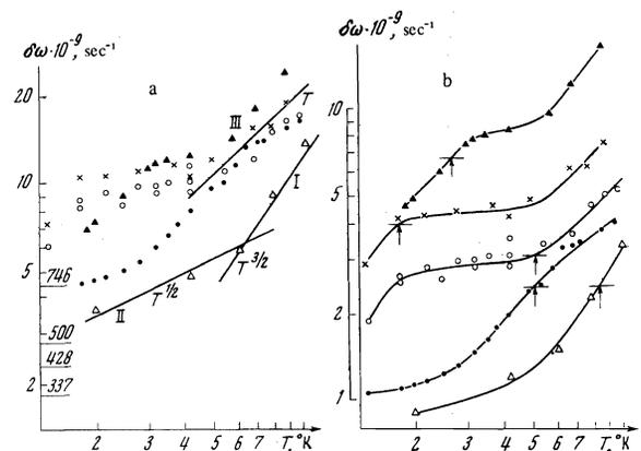
FIG. 2. a) Temperature dependences of  $\delta\omega$  for frequencies  $f$ :  $\Delta$ —131 GHz;  $\bullet$ —337 GHz;  $\circ$ —428 GHz;  $\times$ —500 GHz;  $\blacktriangle$ —746 GHz; the ticks on the axis of ordinates give the values of  $\delta\omega_\infty$  for the corresponding frequencies; b) the same  $\delta\omega(T)$  dependences, along the vertical for clarity. Each curve has an arrow indicating the value  $\delta\omega = 10^{10} \text{ sec}^{-1}$ .
