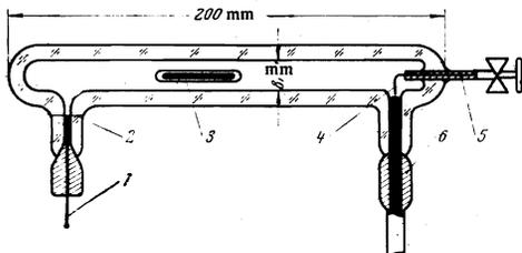
FIG. 1. Piezometer: 1—capillary for introducing mercury, 2—mark indicating the mercury reference level, 3—agitator, 4—electrical lead to the pressure measurement line, 5—capillary for introducing the investigated material, 6—nipple on the pressure measurement line.
