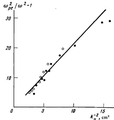
FIG. 7. The function  $\omega_{pe}^2/\omega^2 - 1 = F(k_{||}^2)$ : ●—region I; ○—region III.
