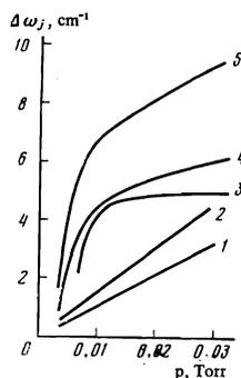
FIG. 4. Pressure dependence of the line widths  $\Delta\omega_1, \Delta\omega_2, \Delta\omega_3$ : The curves correspond to: 1)  $\Delta\omega_1$  without the intense field, 2)  $\Delta\omega_2$  without the intense field, 3)  $\Delta\omega_3$  with the intense field, 4)  $\Delta\omega_2$  with the intense field, 5)  $\Delta\omega_1$  with the intense field.
