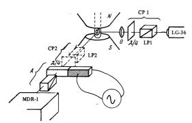
FIG. 2. Experimental setup: CP1 and CP2-circular polarizers, LG-36-helium-neon laser, A-quartz analyzer for the polarized light, MDR-1-spectrometer.
