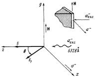
FIG. 1. Experimental geometry used to register the transverse opticalorientation effect. Excitation along the z axis, registration of the recombination radiation along the x axis;  $s_1 = s[1 + (\omega_T T_1)^2]^{-\frac{1}{2}}$ .
