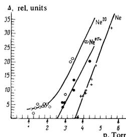
FIG. 6. Measured width of the single-wave generation interval as a function of gas pressure and isotopic composition of the mixture: ●—91% Ne<sup>20</sup> + 9% Ne<sup>22</sup>, +—50% Ne<sup>20</sup> + 50% Ne<sup>22</sup>, ○—98% Ne<sup>20</sup>.
