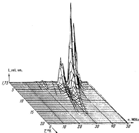
FIG. 3. Temperature dependences of the chlorine NMR signal intensity and frequency in LGC with  $\text{NiCl}_2$ . The intensity scale is relative.
