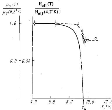
FIG. 3. Temperature dependence of the effective field  $H_{\text{eff}}(T)/H_{\text{eff}}(4.2 \text{ K})$  at the  $\text{Dy}^{3+}$  ion in  $\text{DySb}$ . Solid curve—calculated temperature dependence of the sublattice magnetization (see the text).
