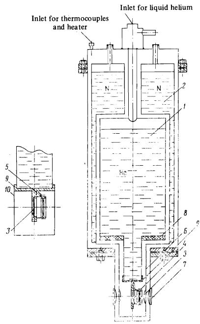
FIG. 1. Helium cryostat. On the left is shown the method used to mount the sample for measurement at temperatures below 4.2°K. 1—helium bath; 2—nitrogen dewar; 3—investigated sample; 4—copper ring with heater; 5—thermal junction; 6—copper screen kept at the temperature of liquid nitrogen; 7—windows of lamsan and aluminum foil; 8—carbon getter; 9—copper holder; 10—additional copper screen.
