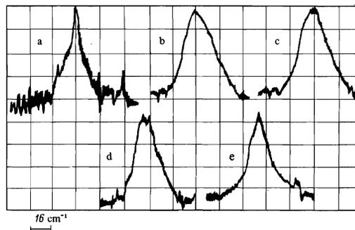
FIG. 5. Emission spectra at input (a) and output (b-e) of the STM under different conditions: a - spectrum of the USP generator,  $\Delta\nu = 5.4 \text{ cm}^{-1}$ ; b - threshold conditions,  $\Delta\nu = 34 \text{ cm}^{-1}$ , c - gain 1.5% above threshold,  $\Delta\nu = 30 \text{ cm}^{-1}$ , d - gain 10% above threshold,  $\Delta\nu = 26 \text{ cm}^{-1}$ , e - gain 15% above threshold,  $\Delta\nu = 20 \text{ cm}^{-1}$ .
