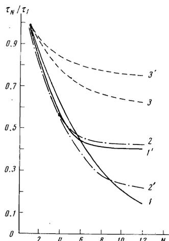
FIG. 4. Calculated dependence of the relative reduction in the pulse length  $\tau_N/\tau_1$  as a function of the number  $N$  of transits through the STM. Curve 1 corresponds to the input signal  $P = P_{th}$ , curve 2 to  $P = 0.5 P_{th}$ , and curve 3 to  $P = 2P_{th}$ . Curves 1', 2', and 3' were obtained for similar input pulses but with STM gain increased by 15% ( $\tau_1$  input pulse length,  $\tau_N$  pulse length after  $N$  transits).
