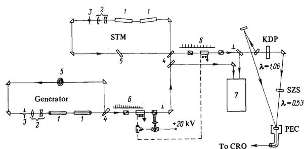
FIG. 1. Block diagram of the apparatus: 1 - active elements (neodymium glass), 2 - compensating lenses, 3 - aperture, 4 - glass wedge, 5 - solution of dye No. 3955 in nitrobenzene, 6 - Pockels shutter, 7 - spectrograph. Initial transmission of dye in generator - 50%, in STM - 15%.
