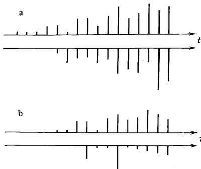
FIG. 8. Variation in the main (a) and scattered (b) radiation in the STM. In case a the scattered radiation was observed through neutral light filters and in case b through SZS-14 and SZS-16 light filters.
