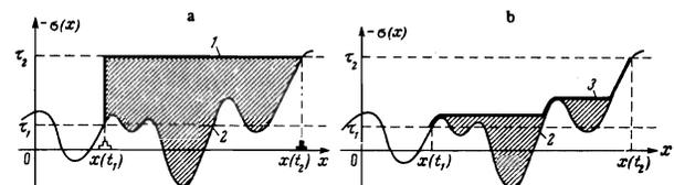
FIG. 1. Energy dissipated when a dislocation moves in a random internal-stress field: a—pulsed loading; b—infinitely slow loading. The heavy lines 1 and 3 show the variation of the external stress along the path of dislocation motion; 2—relief of  $-\sigma(x)$ . The shaded area is equal to the released energy  $W$  divided by the Burgers vector  $b$ .
