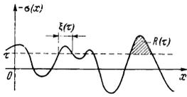
FIG. 3. Spikes of the relief  $-\sigma(x)$  over the level  $\tau$ .  $\xi(\tau)$  is the width of the spike of the relief over this level. The area  $R(\tau)$  of the spike is shown shaded.
