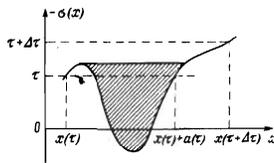
FIG. 2. Change of dislocation mean free path in the case of infinitely slow increases of the external stress from  $\tau$  to  $\tau + \Delta\tau$ . The shaded area is equal to the energy released under such loading, divided by the Burgers vector  $b$ .
