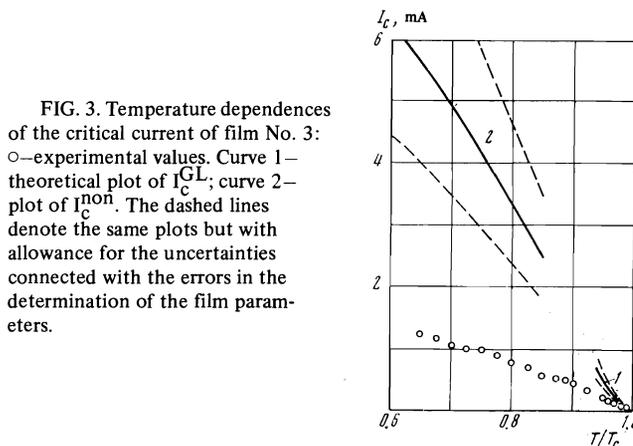
FIG. 3. Temperature dependences of the critical current of film No. 3:  $\circ$ —experimental values. Curve 1— $I_C^{GL}$ ; curve 2—plot of  $I_C^{non}$ . The dashed lines denote the same plots but with allowance for the uncertainties connected with the errors in the determination of the film parameters.
