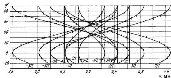
FIG. 2. Experimental values of the resonance frequencies of the  $V^{51}$  satellite NMR transitions in a single crystal of  $V_3Si$  oriented in different ways relative to the applied magnetic field ( $T = 78^\circ K$ ).
