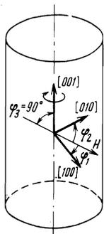
FIG. 1. Position of a sample relative to the applied magnetic field.
